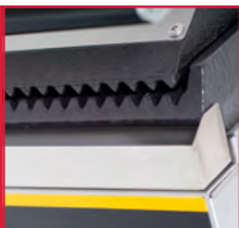
Grease and debris collection gutter
