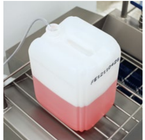
Storage grating for cleaning detergents
