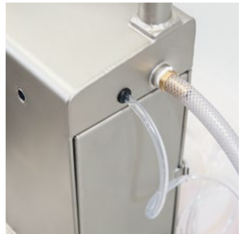
Separate supply of the cleaning detergents
