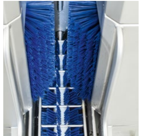
Roller brushes made from nylon
